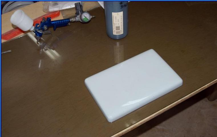
Plug has been sealed, painted, sanded, buffed & coated with mold release
