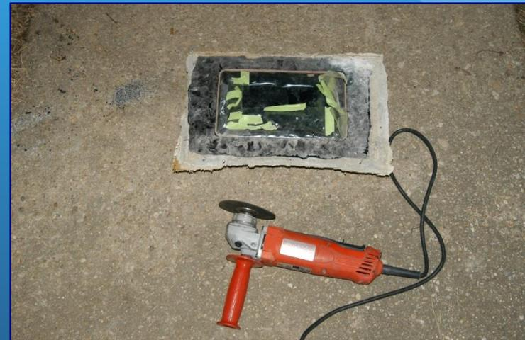
Trim the edges of the mold with a  $\text{AlO}_2$  blade on 4-1/2" grinder
