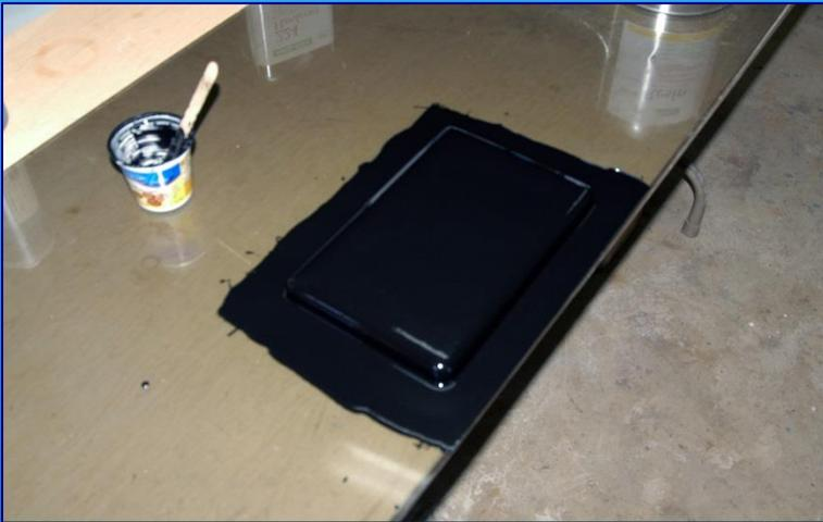
ProSet Tooling Epoxy Applied with to desired thickness. This may require two coats especially on vertical surfaces.
