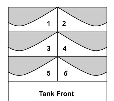
This is how you would lay out the 6 templates on 1/2 sheet of plywood.
