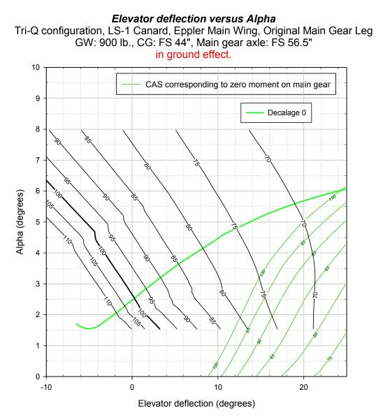
**Figure 19.** Take off relationships for Tri-Q200 (decalage zero). The light green curve represents equilibrium flight configurations. The black contours represent CAS for each configuration. The dark green lines are labeled with CAS which will result in zero weight on the nose wheel (rotation condition). For example, if CAS is constant, increasing elevator deflection will cause the alpha to follow the green curve labeled with that CAS.
