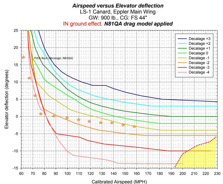
**Figure 10.** Flight configuration curves for equilibrium flight in the Q-2 at 900 pounds GW and CG @ FS 44" in ground effect. Each colored curve represents allowable points for level flight for each decalage value. The yellow stars represent actual flight test measurements from the QAC Q-200 prototype N81QA out of ground effect. Note the difference between modeled flight in ground effect and the stars which were measured outside of ground effect.
