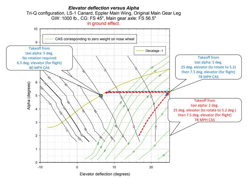
**Figure 21.** Take off relationships for Tri-Q200 (decalage -1). If the taxi ground angle is 5 degrees, the Tri-Q200 will rotate to alpha=5.2 degrees and take off at 78 MPH with elevator at 25 degrees to rotate then reduced to 7.5 degrees for flight. The dashed red curve shows the same transition from taxi angle of alpha=2 degrees
