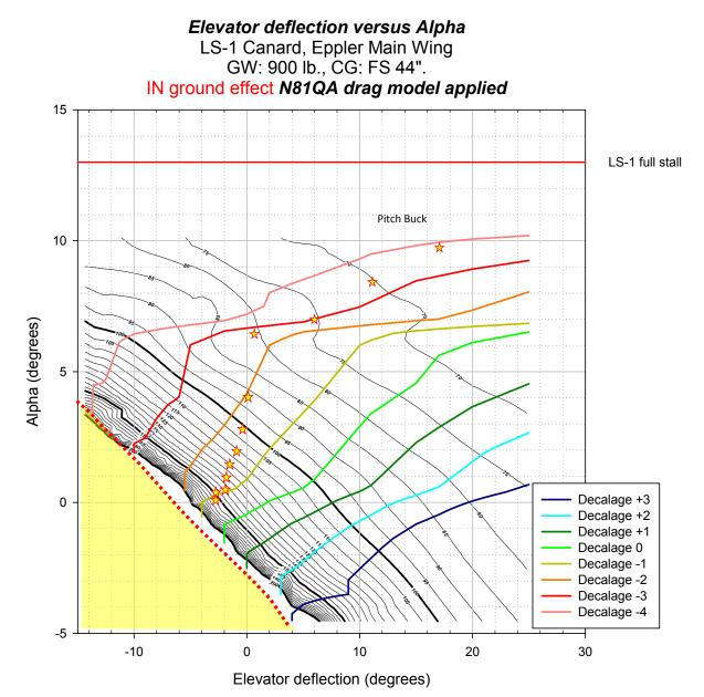
**Figure 9.** Flight configuration curves for equilibrium flight in the Q-2 at 900 pounds GW and CG @ FS 44" in ground effect. Each colored curve represents allowable points for level flight for each decalage value. The yellow stars represent flight test measurements from the QAC Q-200 prototype N81QA outside of ground effect (same as shown on Figure 1). Note the significant difference to Figure 1.
