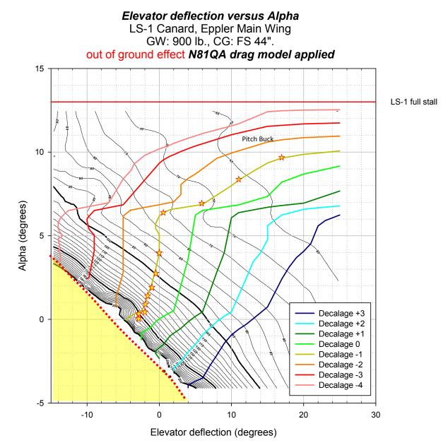
**Figure 1.** Flight configuration curves for equilibrium flight in the Q-2 at 900 pounds GW and CG @ FS 44". Each colored curve represents allowable points for level flight for each decalage value. The results are for flight out of ground effect. The yellow stars represent actual flight test measurements from the QAC Q-200 prototype N81QA. The dotted curve represents the absolute Vne. Flight is likely to be unstable in yellow shaded region. See text for additional explanation.
