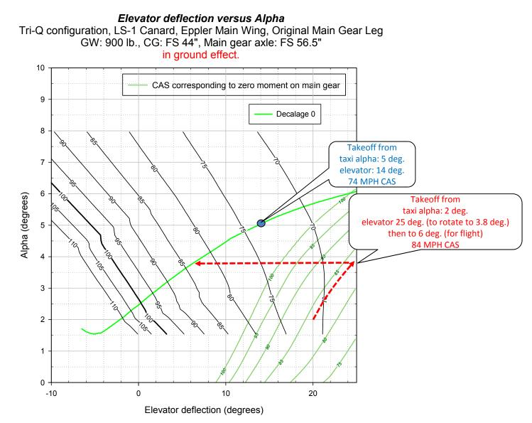
**Figure 20.** Take off relationships for Tri-Q200 (decalage zero). Same as Figure 19. If the taxi ground angle is 5 degrees, the Tri-Q200 will take off at 74 MPH with elevator at 14 degrees (blue dot). The dashed red curve shows transition to take-off at for taxi alpha=2 degrees. 25 deg. elevator to rotate to 3.8 degrees at takeoff, then elevator is reduced to 6 degrees for flight (CAS of 83 MPH).
