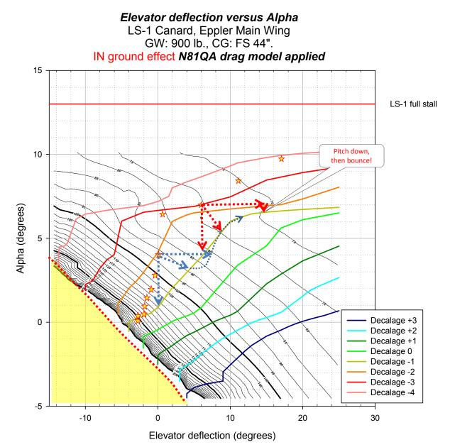
**Figure 12.** Flight configuration curves for equilibrium flight in the Q-2 at 900 pounds GW and CG @ FS 44" in ground effect. Each colored curve represents allowable points for level flight for each decalage value. The yellow stars represent flight test measurements from the QAC Q-200 prototype N81QA out of ground effect. The significance of the blue and red dashed arrow is discussed in detail in the text.
