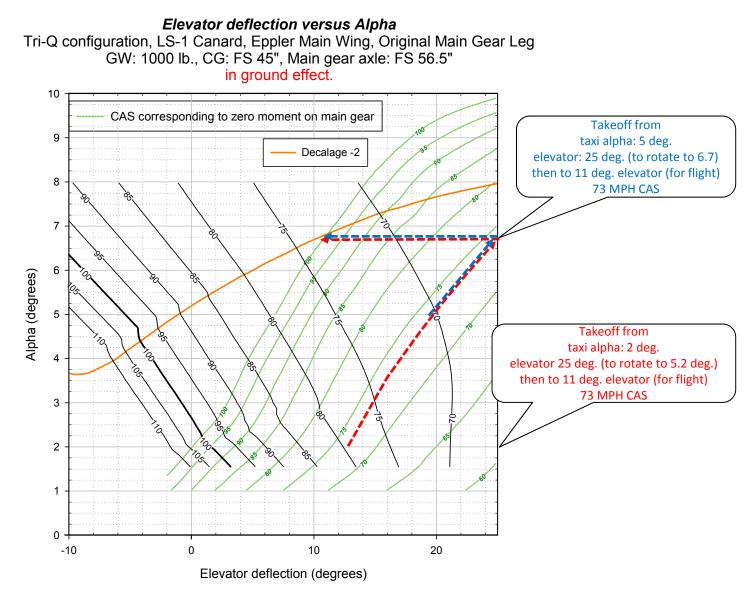
**Figure 22.** Take off relationships for Tri-Q200 (decalage -2). If the taxi ground angle is 5 degrees, the Tri-Q200 will rotate to alpha=6.7 degrees and take off at 73 MPH with elevator at 25 degrees to rotate then reduced to 7.5 degrees for flight. The dashed red curve shows the same transition from taxi angle of alpha=2 degrees
