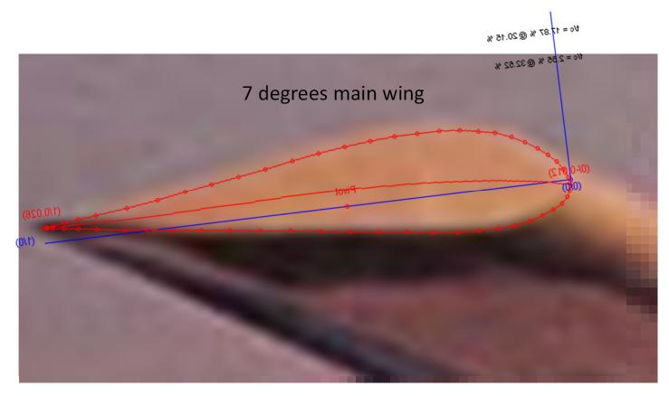
**Figure 3**. Detail of the same historical photo of QAC Q-200 shown in Figure 1. The BL 100 QAC plans template for the Eppler 1212 wing is matched to the photo in the proper location. This indicates that in this photo the Wing is at an 7 degree positive angle in this photo. Since the main wing is at 7 degrees and the canard is at 8 degrees. This photo, as well as other photos confirm that N81QA has a decalage of minus 1.
