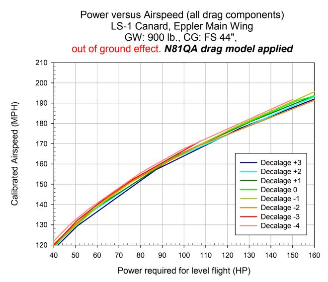
**Figure 8.** Airspeed (CAS) as a function of power (HP) in level flight for the Q-2, LS1 Canard and the N81QA drag model applied. Note that high decalage values of +3 and +2 are the least efficient in the 120-180 CAS range, which decalage values of -3 and -4 decalage are the most efficient. The range is about 6 MPH at 100 HP.
