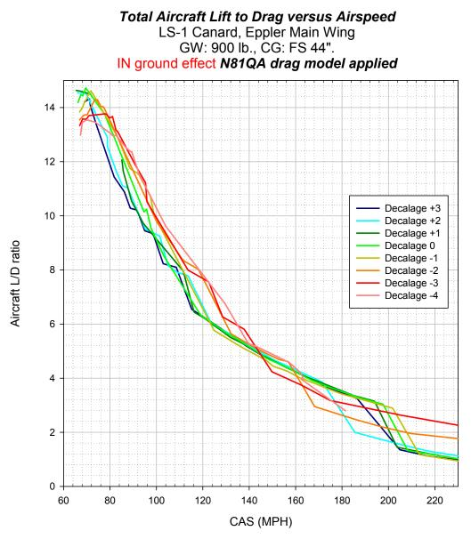
Total Aircraft Lift to Drag (L/D) vs Airspeed (CAS) for the N81QA Q-200 model. The range of decalage modeled is -4 to +3. These curves represent response in ground effect.
