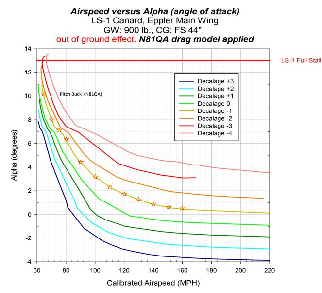
**Figure 12.** Airspeed versus alpha curves for equilibrium flight in the Q-2 at 900 pounds GW and CG @ FS 44" Each colored curve represents allowable points for level flight for each decalage value. The results are for flight out of ground effect. The yellow stars represent actual flight test measurements from the QAC Q-200 prototype N81QA. The blue stars represent the estimated flight test data points from video analysis of a similarly loaded Tri-Q 200 with a decalage of minus 0.4 degrees.
