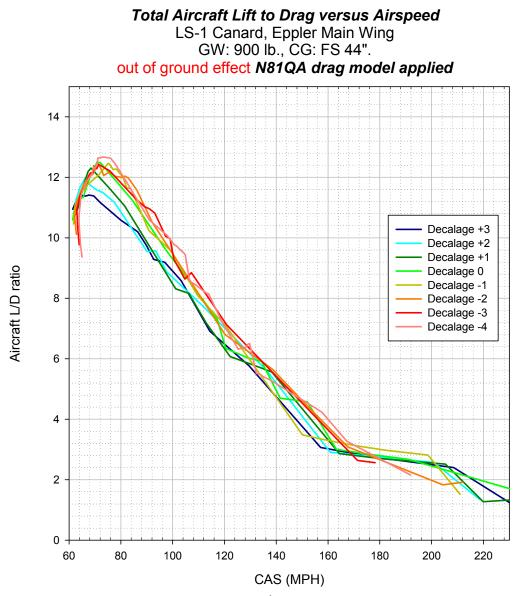
**Figure 6.** Total Aircraft Lift to Drag (L/D) vs Airspeed (CAS) for the N81QA Q-200 model. The range of decalages modeled is -4 to +3. All decalage models show max L/D below 80 mph CAS, with decalage of -2 and -1 very below 70 MPH. The decalage of +3 has a minimum glide angle near 65 mph. Decalage of 0 (plans built) achieves the highest L/D, of 12.5at 72 mph CAS.`
