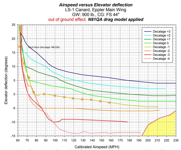
**Figure 4.** Flight configuration curves for equilibrium flight in the Q-2 at 900 pounds GW and CG @ FS 44" Each colored curve represents allowable points for level flight for each decalage value. The results are for flight out of ground effect. The yellow stars represent actual flight test measurements from the QAC Q-200 prototype N81QA. The dotted curve represents the absolute Vne. Stable flight not possible in yellow shaded region.
