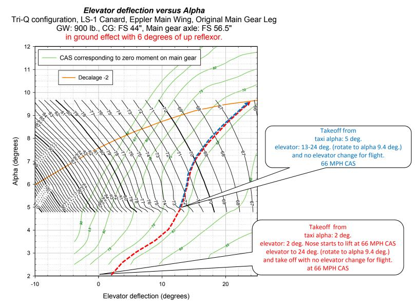
**Figure 23.** Take off relationships for Tri-Q200 (decalage -2) with reflexor set to 6 degrees trailing edge up. If the taxi ground angle is 5 degrees, the Tri-Q200 will rotate to alpha=9.4 degrees and take off at 66 MPH with elevator at 24 degrees. The dashed red curve shows the same transition from taxi angle of alpha=2 degrees. The dashed blue curve shows transition from taxi alpha of 5 degrees
