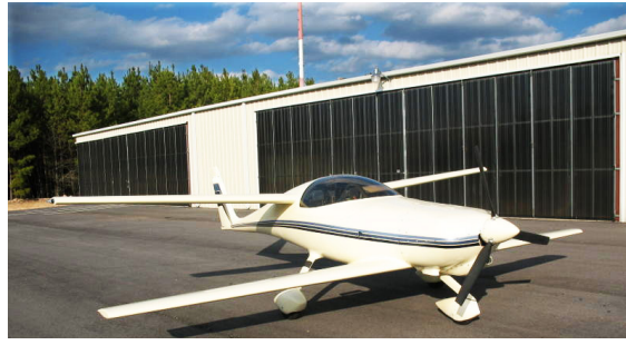
Figure 1. Example tandem wing aircraft, a Tri-Q200.
