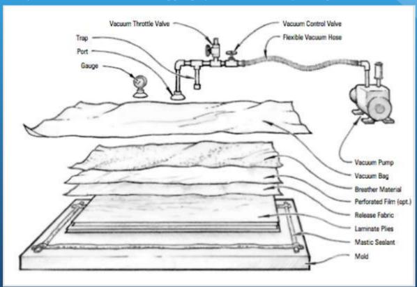
Vacuum assisted system would have a resin source opposite of the vacuum source (TYP)
