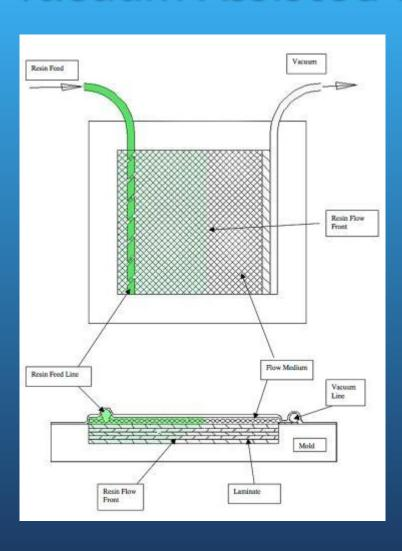
Very basic layout of the process. The supporting equipment for this procedure is not shown here.
