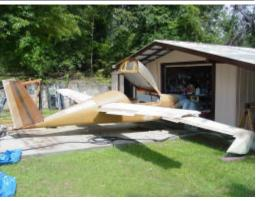
$2^{nd}$  project is a standard Dragonfly built from plans. Fuselage sides & belly pan and bulkheads done, wing completed, and all foam for rest of plane is cut ready to glass, all glass to finish and carbon fiber included, nearly complete Ken Brock metal control kits, Fiberglass hoop gear, wheel and tires, brakes, + more,
