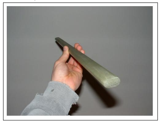
Now that is a nice looking tail spring Joe!!! Joe has come up with a very easy way to lay-up his own tail spring that could be duplicated by any of us. This is exactly how I laid up my main gear. Something I found very useful was to wet out the glass outside the mold on the bench. It was very easy to get the glass wetted out and very easy to remove the excess epoxy.
