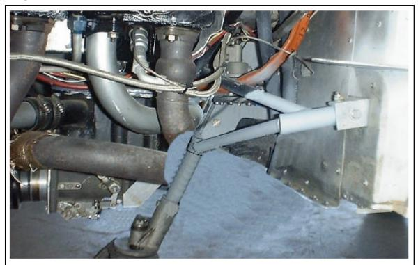
View of the new support tube welded to the motor mount
