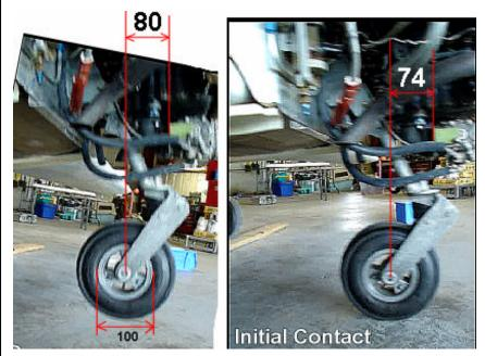
tion showed the gear moved to the side about <sup>1</sup>/<sub>4</sub> inches and stayed there. Dropping the gear from the other direction straightened it out but that just meant something was moving. The test showed that the aluminum brackets we used to deliver the loads to the firewall were stronger than the firewall and the holes were elongating.
