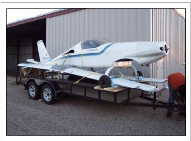
Here is Mark's Dragonfly loaded up and ready for the trip back to Alabama. You might notice the engine is still installed on the plane. In the past many people have commented about removing or supporting the engine prior to ground transport. Mark's plane was not damaged on this trip, but I would recommend that you either remove or support your engine during ground transport.
