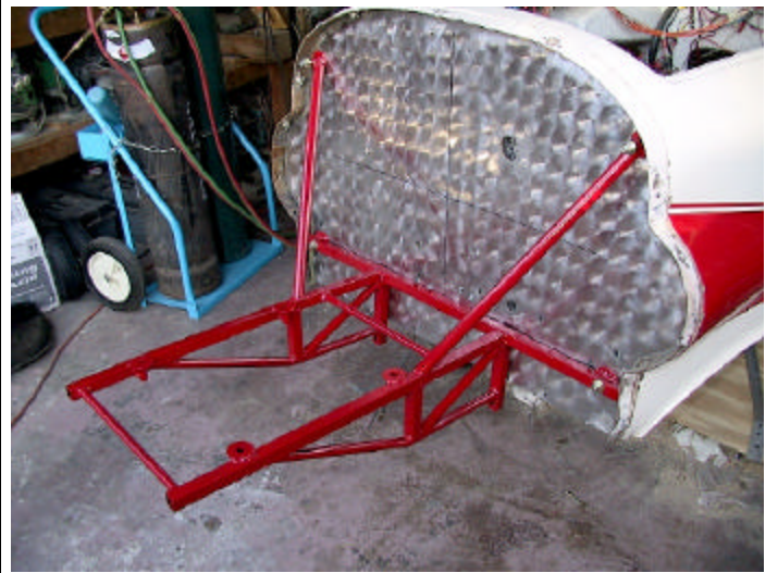
An engine mount of my design, mounted to the firewall of the Dragonfly I bought from Don Stewart, which was built by the late Rob Roe.
