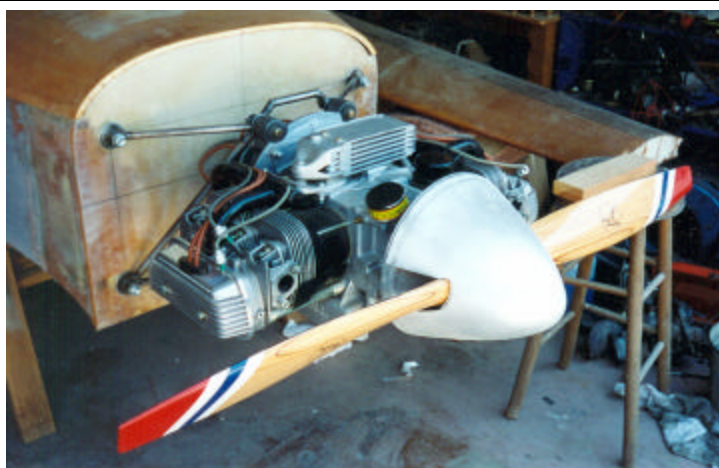
The firewall was modified for the "new style" mount and the HAPI engine was hung when I decided to go Corvair.
