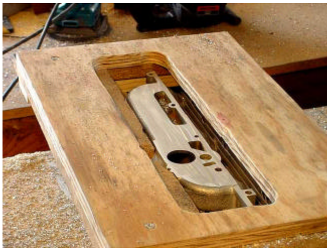
Using a plywood fixture and a 3hp, 1/2" shank router with a 1" diameter straight flute carbide bit, I was able to mill the carburetor mounting boss off the top of the stock cast intake log, to keep the intake runners profile very low.
