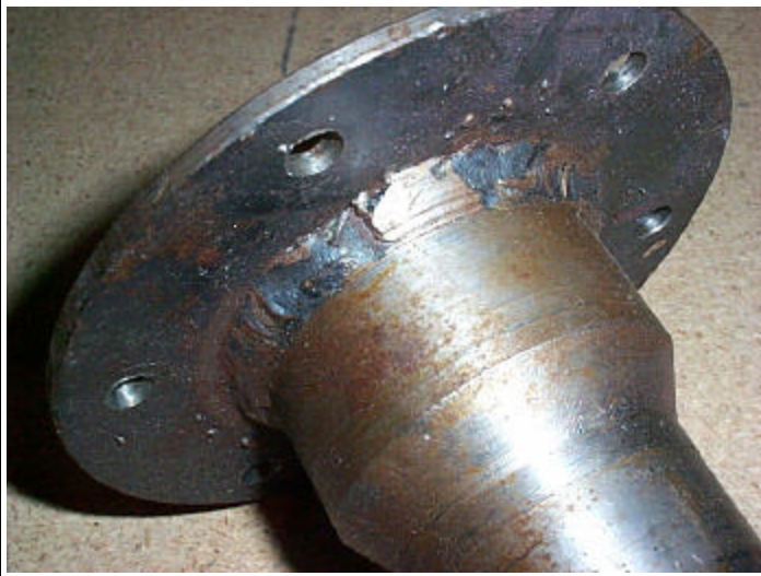
This shot of the prop hub is one small example of the poor quality of the “converted” engine I got for $500. Let the buyer beware.
