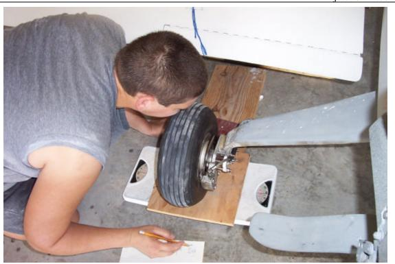
Drew weighs his landing gear on a pair of bathroom scales.
