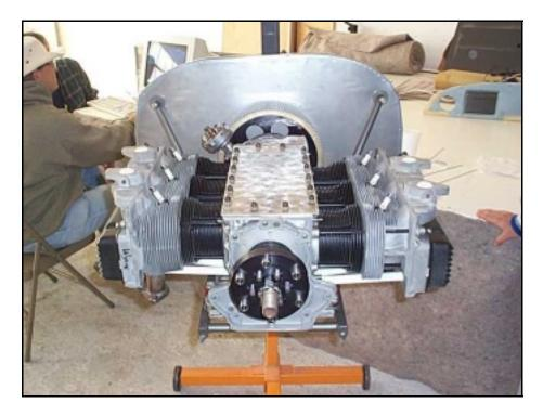
William Wynne's 3100cc 6 cylinder Corvair engine. In smaller trim (2700cc) this engine produces a reliable, honest 100 hp @ 3200 rpm, and weighs in at under 250 lbs all up. This actual engine is highly experimental. It will be turbocharged, and should make 140hp or better, at altitude.
