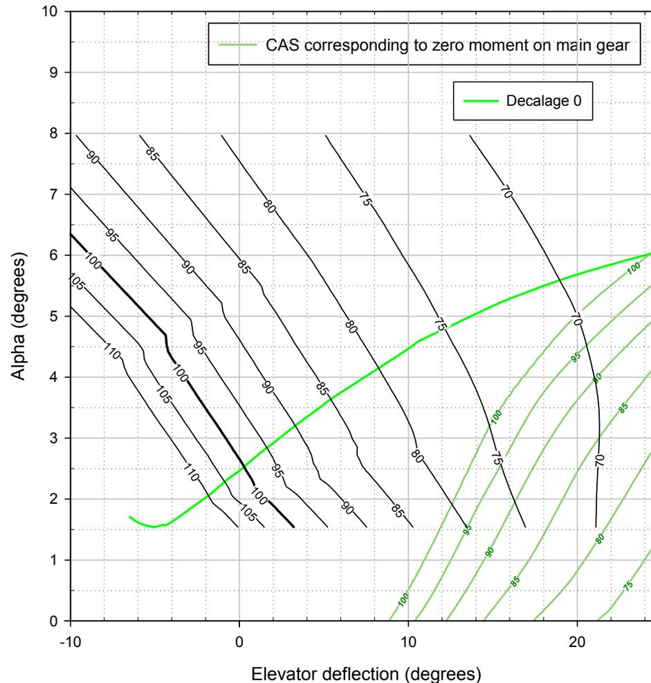
**Figure 19.** Take off relationships for Tri-Q200 (decalage zero). The light green curve represents equilibrium flight configurations. The black contours represent CAS for each configuration. The dark green lines are labeled with CAS which will result in zero weight on the nose wheel (rotation condition). For example, if CAS is constant, increasing elevator deflection will cause the alpha to follow the green curve labeled with that CAS.
