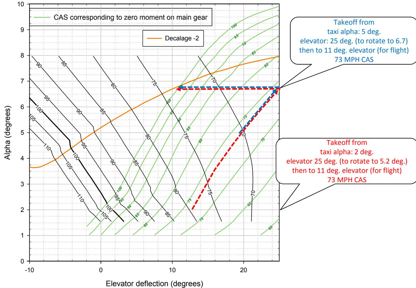
**Figure 22.** Take off relationships for Tri-Q200 (decalage -2). If the taxi ground angle is 5 degrees, the Tri-Q200 will rotate to alpha=6.7 degrees and take off at 73 MPH with elevator at 25 degrees to rotate then reduced to 7.5 degrees for flight. The dashed red curve shows the same transition from taxi angle of alpha=2 degrees
