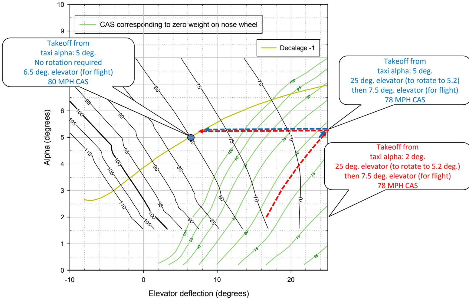
**Figure 21.** Take off relationships for Tri-Q200 (decalage -1). If the taxi ground angle is 5 degrees, the Tri-Q200 will rotate to alpha=5.2 degrees and take off at 78 MPH with elevator at 25 degrees to rotate then reduced to 7.5 degrees for flight. The dashed red curve shows the same transition from taxi angle of alpha=2 degrees
