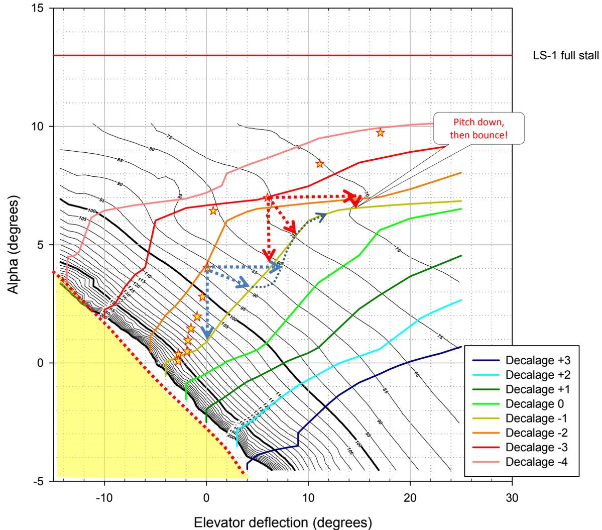
**Figure 12.** Flight configuration curves for equilibrium flight in the Q-2 at 900 pounds GW and CG @ FS 44" in ground effect. Each colored curve represents allowable points for level flight for each decalage value. The yellow stars represent flight test measurements from the QAC Q-200 prototype N81QA out of ground effect. The significance of the blue and red dashed arrow is discussed in detail in the text.
