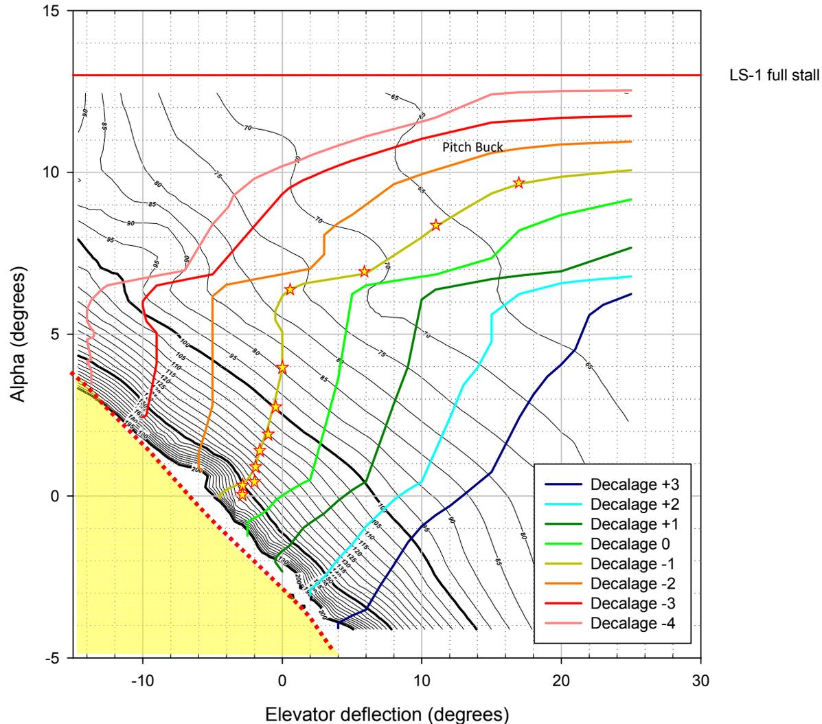
**Figure 1.** Flight configuration curves for equilibrium flight in the Q-2 at 900 pounds GW and CG @ FS 44". Each colored curve represents allowable points for level flight for each decalage value. The results are for flight out of ground effect. The yellow stars represent actual flight test measurements from the QAC Q-200 prototype N81QA. The dotted curve represents the absolute Vne. Flight is likely to be unstable in yellow shaded region. See text for additional explanation.
