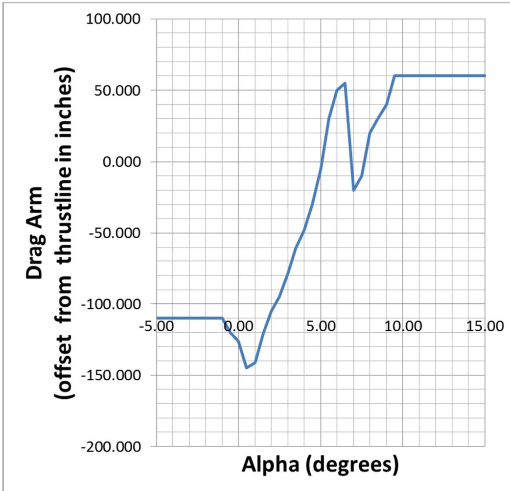
**Figure 5.** Lift-independent non-wing drag moment-arm vs. Alpha model applied to Javafoil model. This variable arm model is required to cause the elevator deflections and airspeeds in the model to match the actual N81QA flight test data. Negative values of drag arm mean that the arm is below the thrust line, resulting in a forward pitching moment. The drag force applied to this arm is computed from the standard drag formula so is proportional to the square of airspeed.
