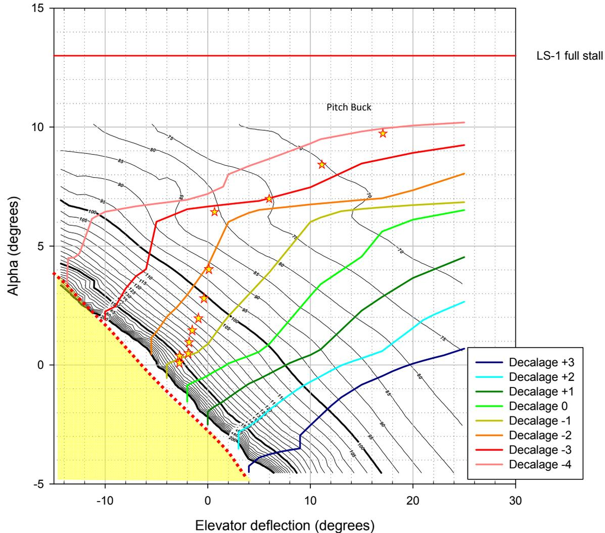
**Figure 9.** Flight configuration curves for equilibrium flight in the Q-2 at 900 pounds GW and CG @ FS 44" in ground effect. Each colored curve represents allowable points for level flight for each decalage value. The yellow stars represent flight test measurements from the QAC Q-200 prototype N81QA outside of ground effect (same as shown on Figure 1). Note the significant difference to Figure 1.
