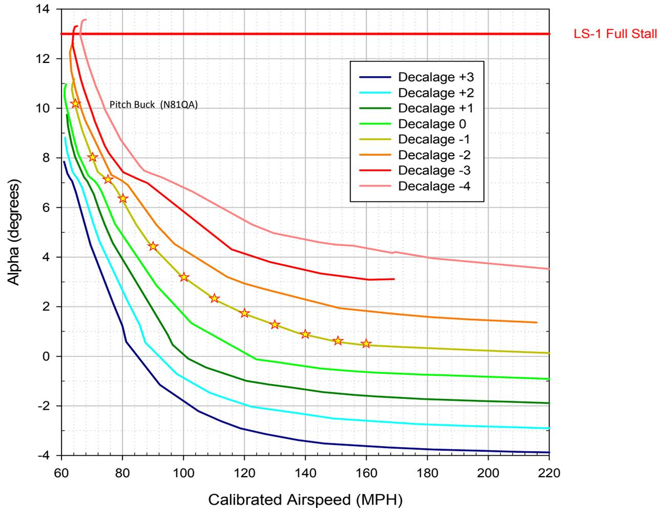
**Figure 12.** *Airspeed versus alpha curves for equilibrium flight in the Q-2 at 900 pounds GW and CG @ FS 44"*
