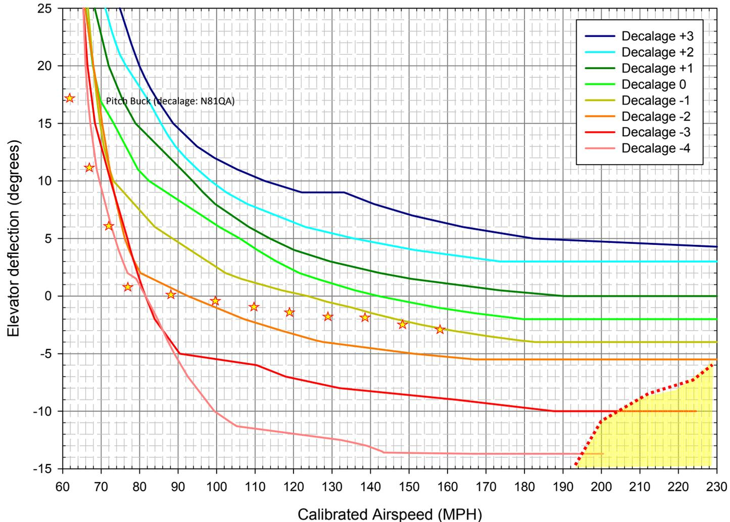
**Figure 10.** Flight configuration curves for equilibrium flight in the Q-2 at 900 pounds GW and CG @ FS 44" in ground effect. Each colored curve represents allowable points for level flight for each decalage value. The yellow stars represent actual flight test measurements from the QAC Q-200 prototype N81QA out of ground effect. Note the difference between modeled flight in ground effect and the stars which were measured outside of ground effect.
