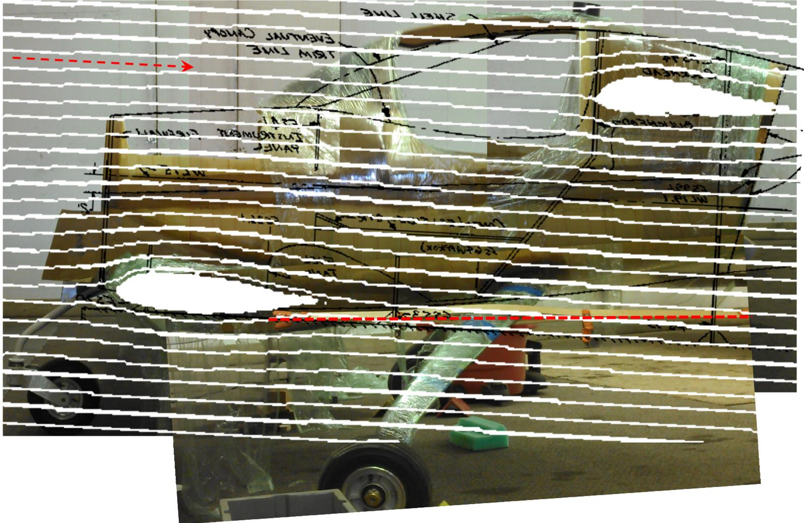
**Figure 15.** Measurement of mean chord of the outer part the main gear leg's mean chord angle (red dashed curve) versus Javafoil streamlines (white) laid over partially built Tri-Q2. The red line makes a negative 8 degree angle to the relative wind when the aircraft is flying at Alpha=0 .
