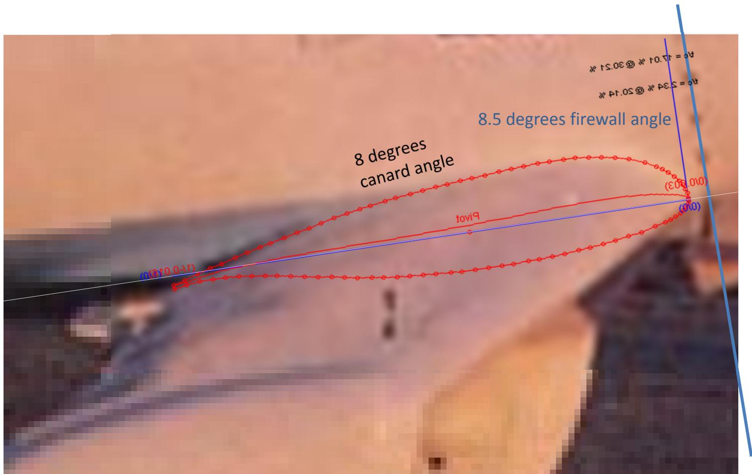
**Figure 2.** Detail of historical photo of QAC Q-200 Prototype N81QA. The BL 15 QAC plans template for the LS-1 canard is matched to the photo in the proper location. This indicates that in this photo the Canard is at an 8 degree positive angle in this photo, and the firewall is slightly higher at about 8.5 degrees.
