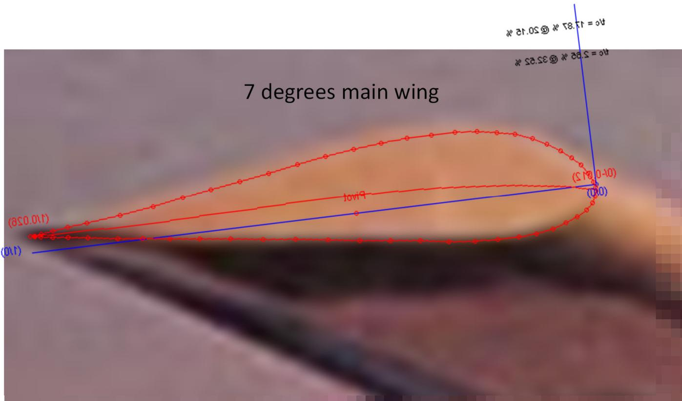
**Figure 3.** Detail of the same historical photo of QAC Q-200 shown in Figure 1. The BL 100 QAC plans template for the Eppler 1212 wing is matched to the photo in the proper location. This indicates that in this photo the Wing is at an 7 degree positive angle in this photo. Since the main wing is at 7 degrees and the canard is at 8 degrees. This photo, as well as other photos confirm that N81QA has a decalage of minus 1.
