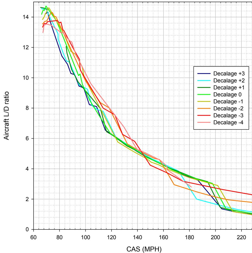
Total Aircraft Lift to Drag (L/D) vs Airspeed (CAS) for the N81QA Q-200 model. The range of decalage modeled is -4 to +3. These curves represent response in ground effect.
