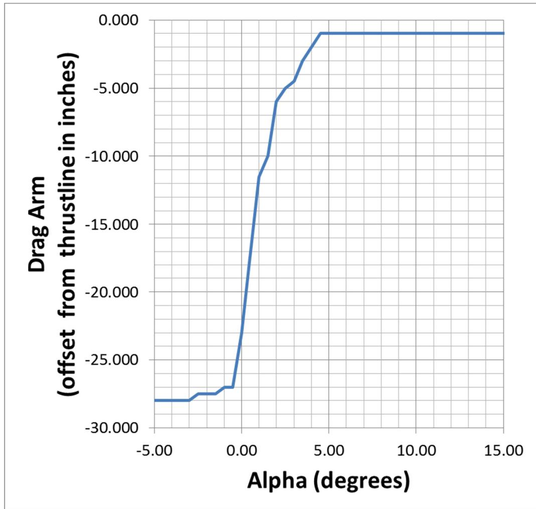
**Figure 18.** Lift-independent non-lift drag moment-arm vs. Alpha model for the Tri-Q200 applied to Javafoil model. This model is typical of that expected for the Tri-Q200 where the gear leg drags are all located below the thrust. The drag force applied to this arm is computed from the drag formula so is proportional to the square of airspeed.
