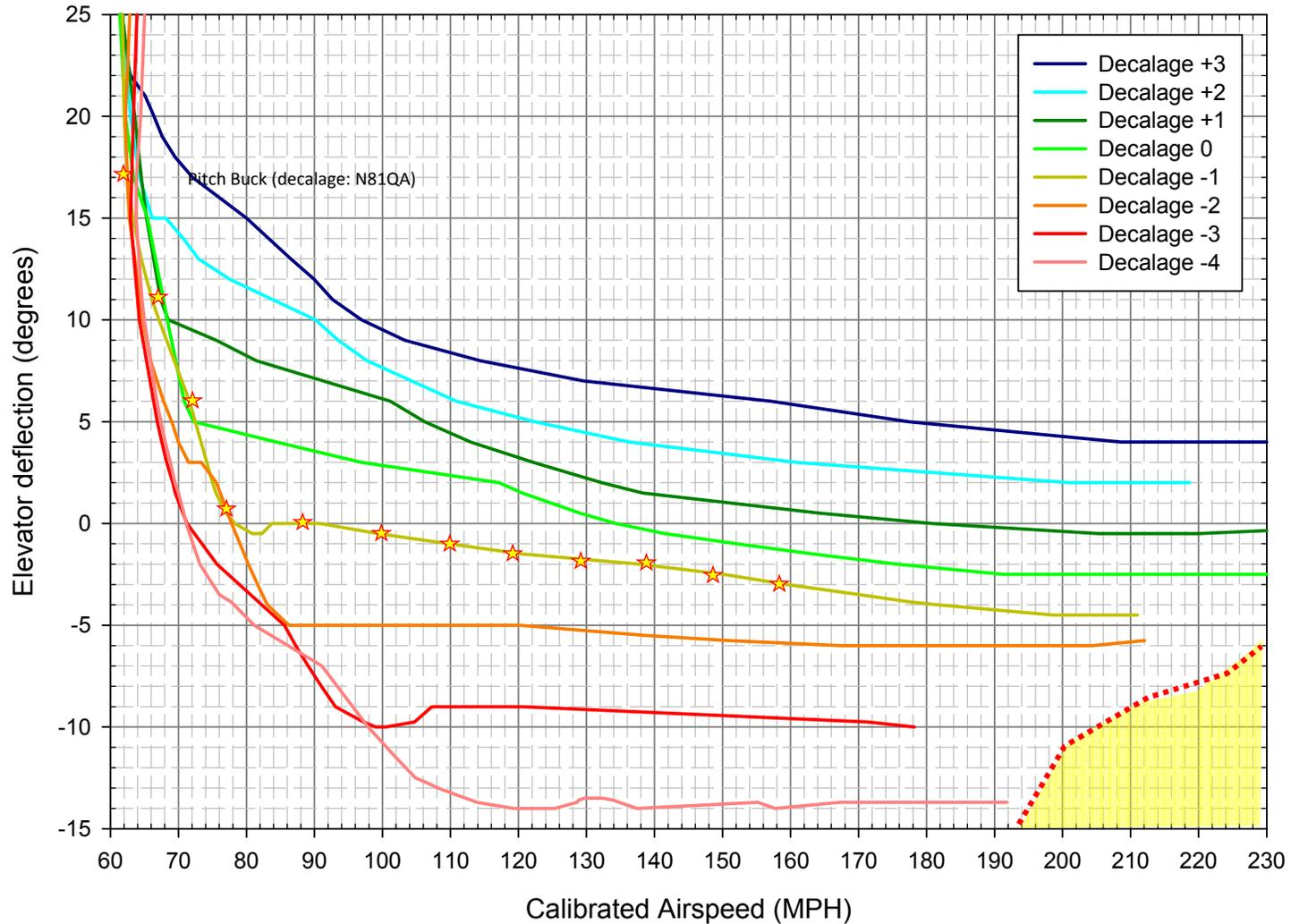
**Figure 4.** Flight configuration curves for equilibrium flight in the Q-2 at 900 pounds GW and CG @ FS 44"
