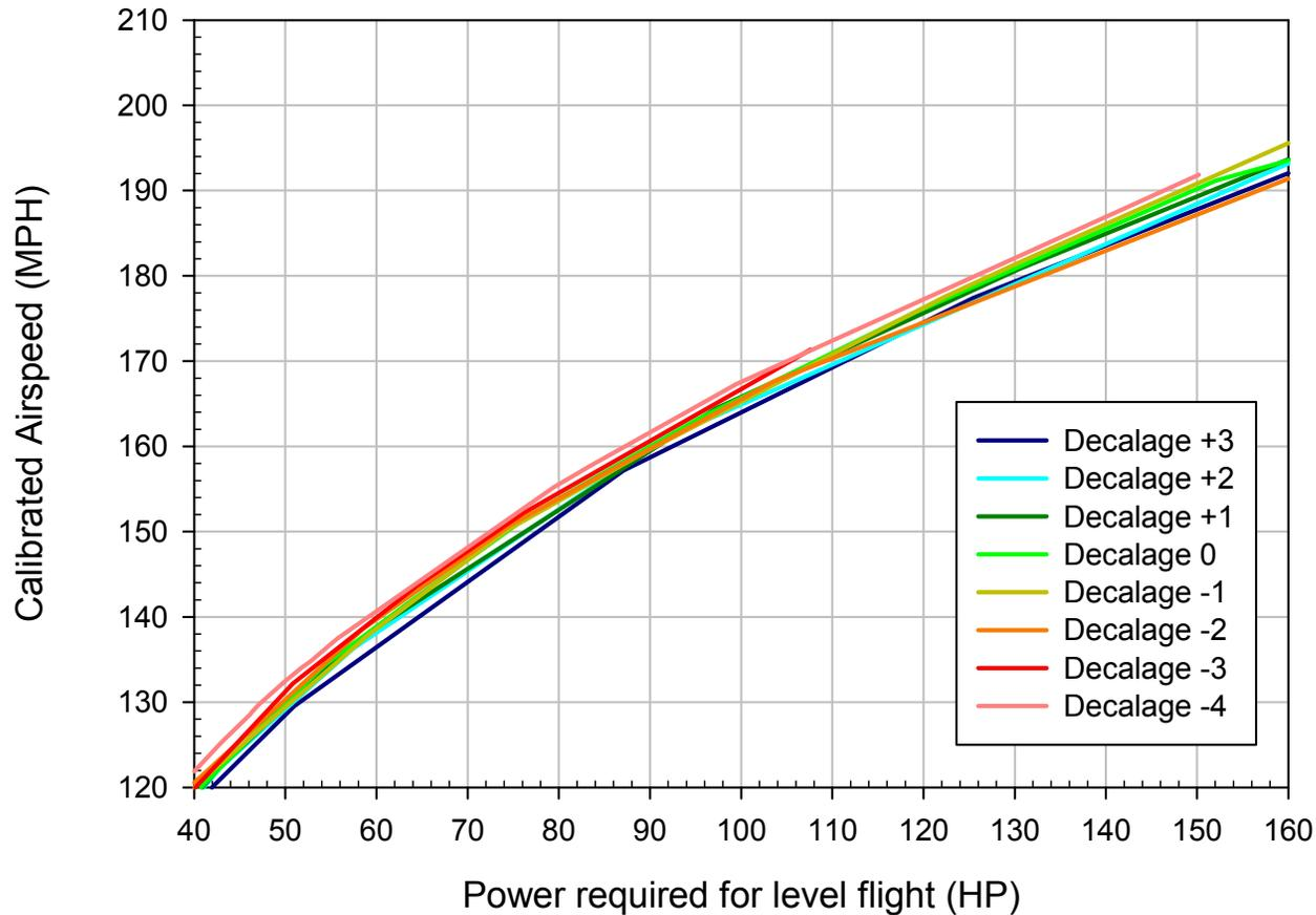
**Figure 8.** Airspeed (CAS) as a function of power (HP) in level flight for the Q-2, LS1 Canard and the N81QA drag model applied. Note that high decalage values of +3 and +2 are the least efficient in the 120-180 CAS range, which decalage values of -3 and -4 decalage are the most efficient. The range is about 6 MPH at 100 HP.
