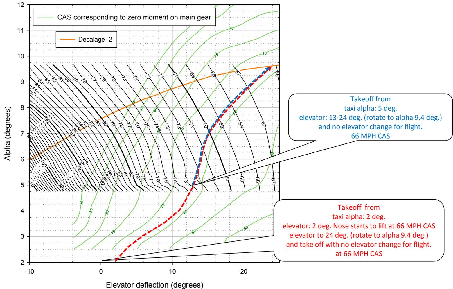
**Figure 23.** Take off relationships for Tri-Q200 (decalage -2) with reflexor set to 6 degrees trailing edge up. If the taxi ground angle is 5 degrees, the Tri-Q200 will rotate to alpha=9.4 degrees and take off at 66 MPH with elevator at 24 degrees. The dashed red curve shows the same transition from taxi angle of alpha=2 degrees. The dashed blue curve shows transition from taxi alpha of 5 degrees
