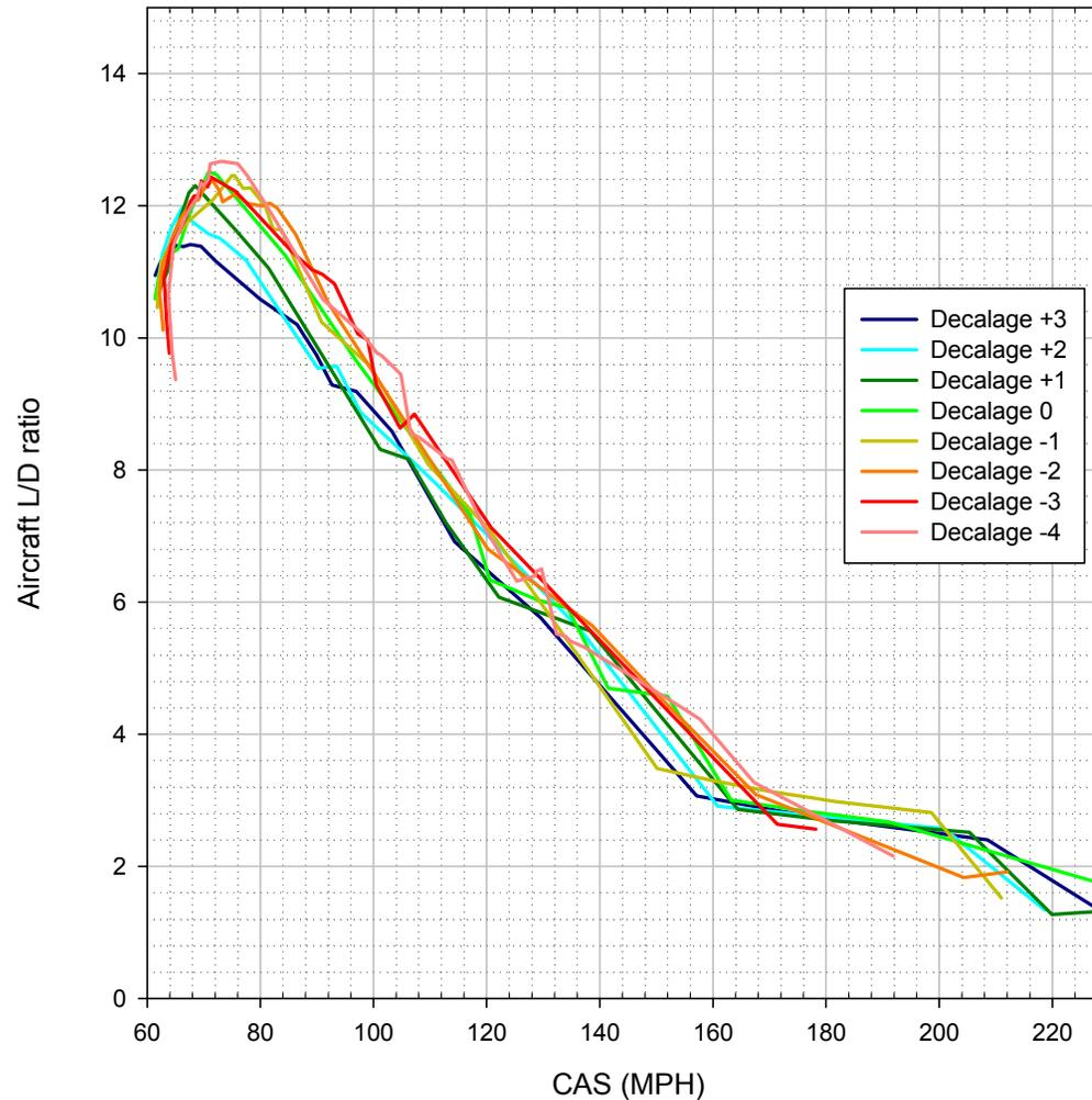
**Figure 6.** Total Aircraft Lift to Drag (L/D) vs Airspeed (CAS) for the N81QA Q-200 model. The range of decalages modeled is -4 to +3. All decalage models show max L/D below 80 mph CAS, with decalage of -2 and -1 very below 70 MPH. The decalage of +3 has a minimum glide angle near 65 mph. Decalage of 0 (plans built) achieves the highest L/D, of 12.5 at 72 mph CAS.
