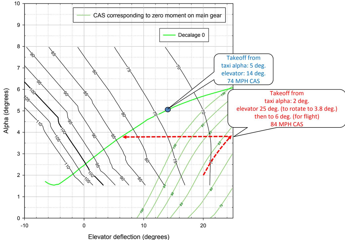
**Figure 20.** Take off relationships for Tri-Q200 (decalage zero). Same as Figure 19. If the taxi ground angle is 5 degrees, the Tri-Q200 will take off at 74 MPH with elevator at 14 degrees (blue dot). The dashed red curve shows transition to take-off at for taxi alpha=2 degrees. 25 deg. elevator to rotate to 3.8 degrees at takeoff, then elevator is reduced to 6 degrees for flight (CAS of 83 MPH).
