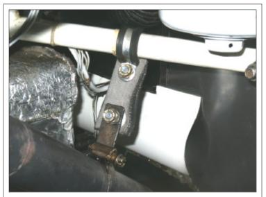
ting the plane ready for flight the exhaust pipe hangers were overlooked. A few hours into his test flight program he told me the plane was making a funny noise and he found a piece of one of the pipes had broken off and the pipes were cracked at the last weld. After repairs to the pipes, he constructed and installed hangers and has had no further problems.
