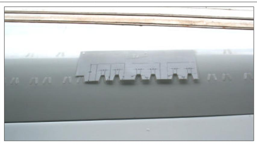
In the photo with the template there are three of the original templates copied and laminated to one large sheet. This makes it very easy to keep the VG's aligned. The amount of VG's installed is about 40 short of the recommended amount. At this point I don't know if the addition of those will produce more lift or add drag but I am very happy with the effects these VG's produce mounted at the 50% cord line. This is the template I made to ensure consistent spacing.
