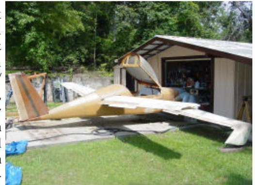
2<sup>nd</sup> project is a standard Dragonfly built from plans. Fuselage sides & belly pan and bulkheads done, wing completed, and all foam for rest of plane is cut ready to glass, all glass to finish and carbon fiber included, nearly complete Ken Brock metal control kits, Fiberglass hoop gear, wheel and tires, brakes, + more,
