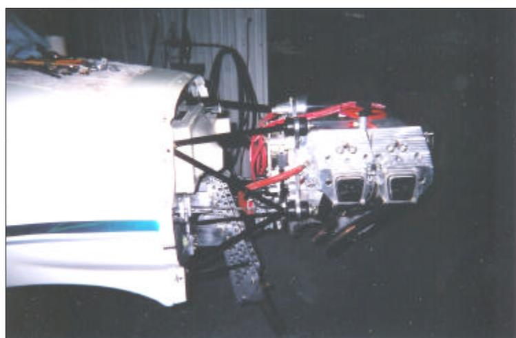
The flight went off without any problems and only a minor elevator adjustment was required to correct a heavy wing condition. The plane has the Jabiru 2200 installed and the nose wheel is from a BD-5. Joe is currently looking for a new more heavy duty nose wheel because the BD-5 unit is not quite up to the task. The plane currently tips the scales at 705 pounds.
