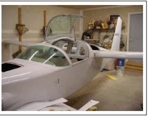
canard was set too low and his wing was set to high. In simulation, the plane required almost full down elevator during take-off and generally did not fly as it should. Joe decided to bite the bullet and adjust the wing install angle as much as he could. He is in the process of installing a reflexor system like Patrick Hildebrand's as featured in DBFN #100.
