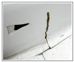
fracture appeared on the outside as well as the inside of the fuselage. This area is one of the strongest areas of the fuselage and it had gone through a failure mode similar to attempting to open as if it were the front of a C5A, or that pregnant Airbus that appeared a OSH this year. On the top of the front turtle deck, there was a rip extending from the front right corner of the access panel forward to the right approaching the firewall.
