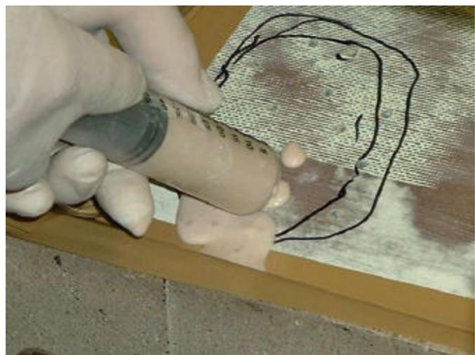
**Injecting the slurry**
