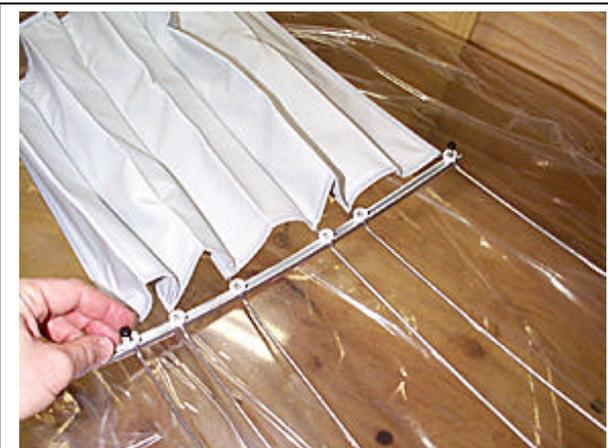
*Upper left photo shows the business side of the center aluminum channel, which the bows ride upon. Double sided tape (shown orange) adheres the track to the canopy. The photo at the left shows the shade installed on one side of the rail and the wire ribs on the other. Mystery hand points to the thumb screw that locks the shade in the extend position. Van's has been flying the SunShade on their aircraft for some time now and seem to be pleased with the performance of the shade.*
